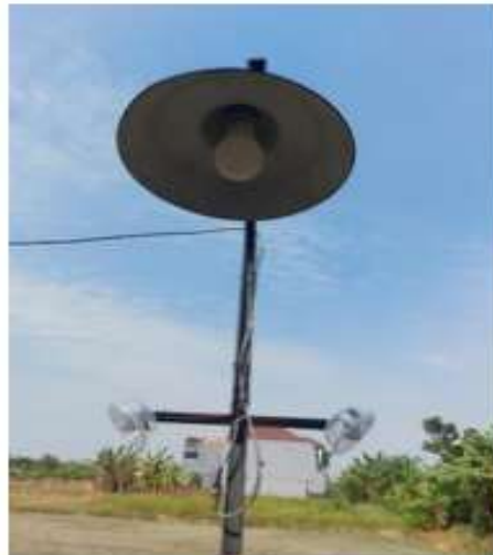
Figure 5. Realized PJU lamp pole and PIR sensor modules
