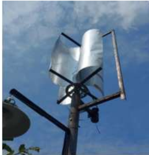
Figure 3. Realized four-blade Savonius turbine and DC generator
